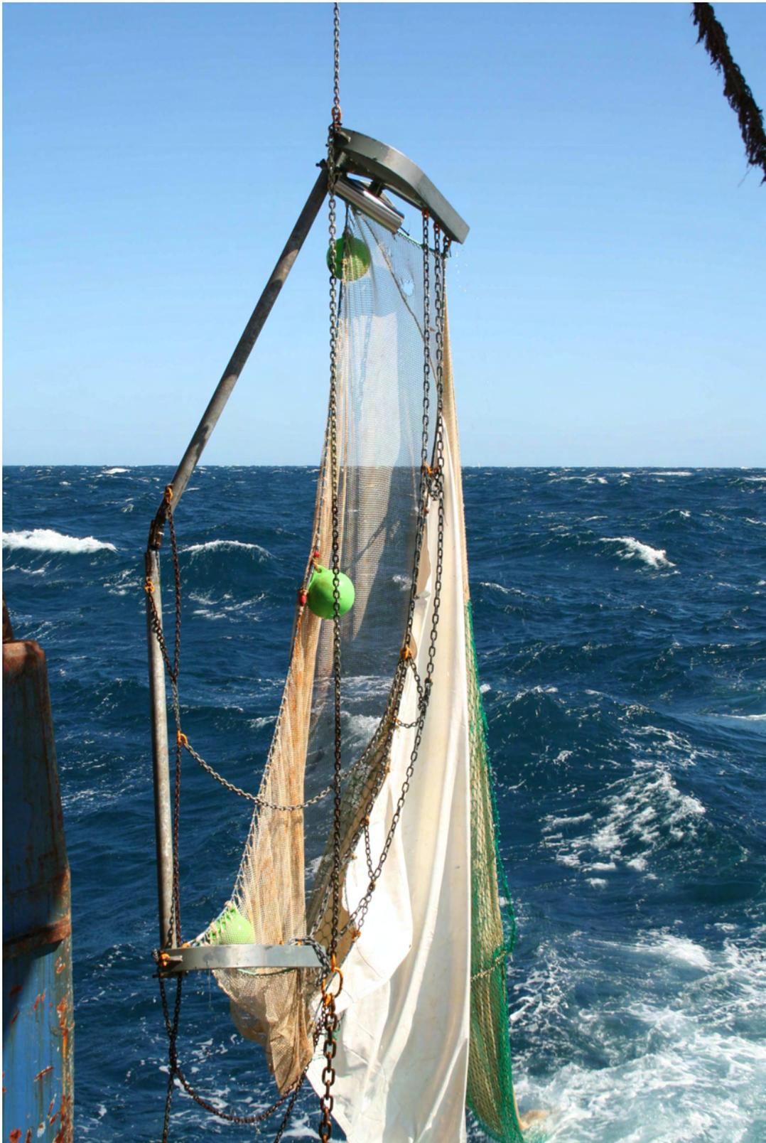
Figure 3: The beam very bent. Note the torn aluminium plug used as a weak link.
